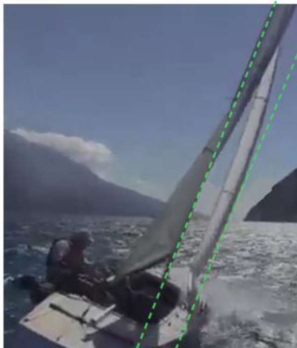
Figure 14 Jib tuning: Leech parallel to the mast
