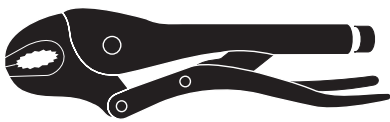
Wrench for flats on upper stud of turnbuckle or needle nose vise-grip-type pliers if there are no wrench flats
