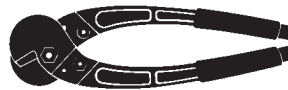
Wire cutters - only needed if you are cutting your own headstay wire
