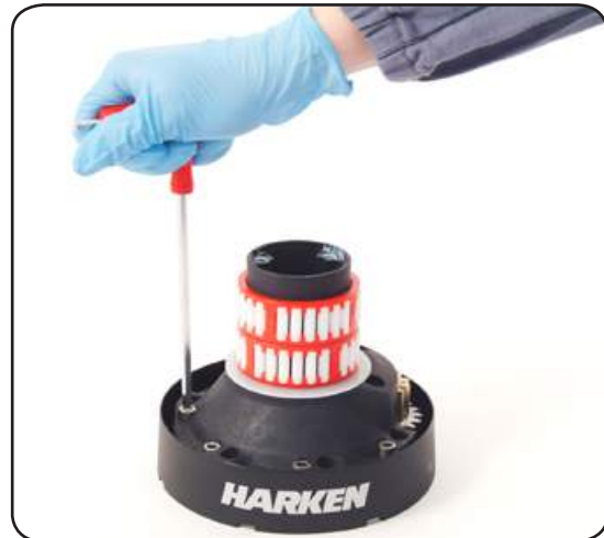
9. Unscrew the 6 hex screws n°16 (8Nm/71 in-lb)
