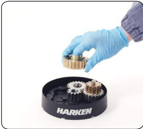
12. Remove the gearing n°7 and remove the pawls n°5. To facilitate the operation press the spring against the pawl with a blade.
