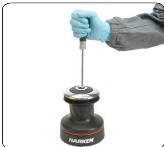
1. Unscrew the central screw ( \approx 2\text{Nm}/18\text{ in-lb} )
