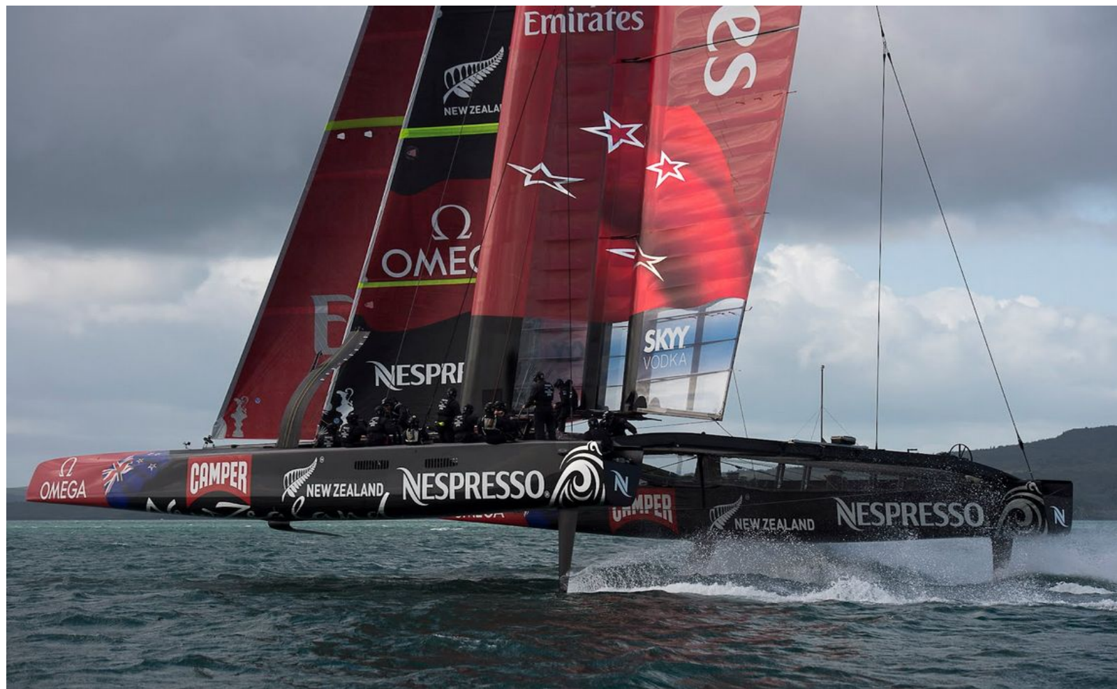
Emirates New Zealand - AC72 2013 (22m) Hydrofoil catamaran note the C-Z shaped foil and the rigid wing hydraulic controlled.
