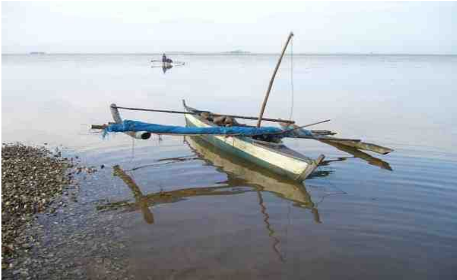
Philippine Fisherman Canoe, note the two outrigger stabilizers. Multi-hull design!
