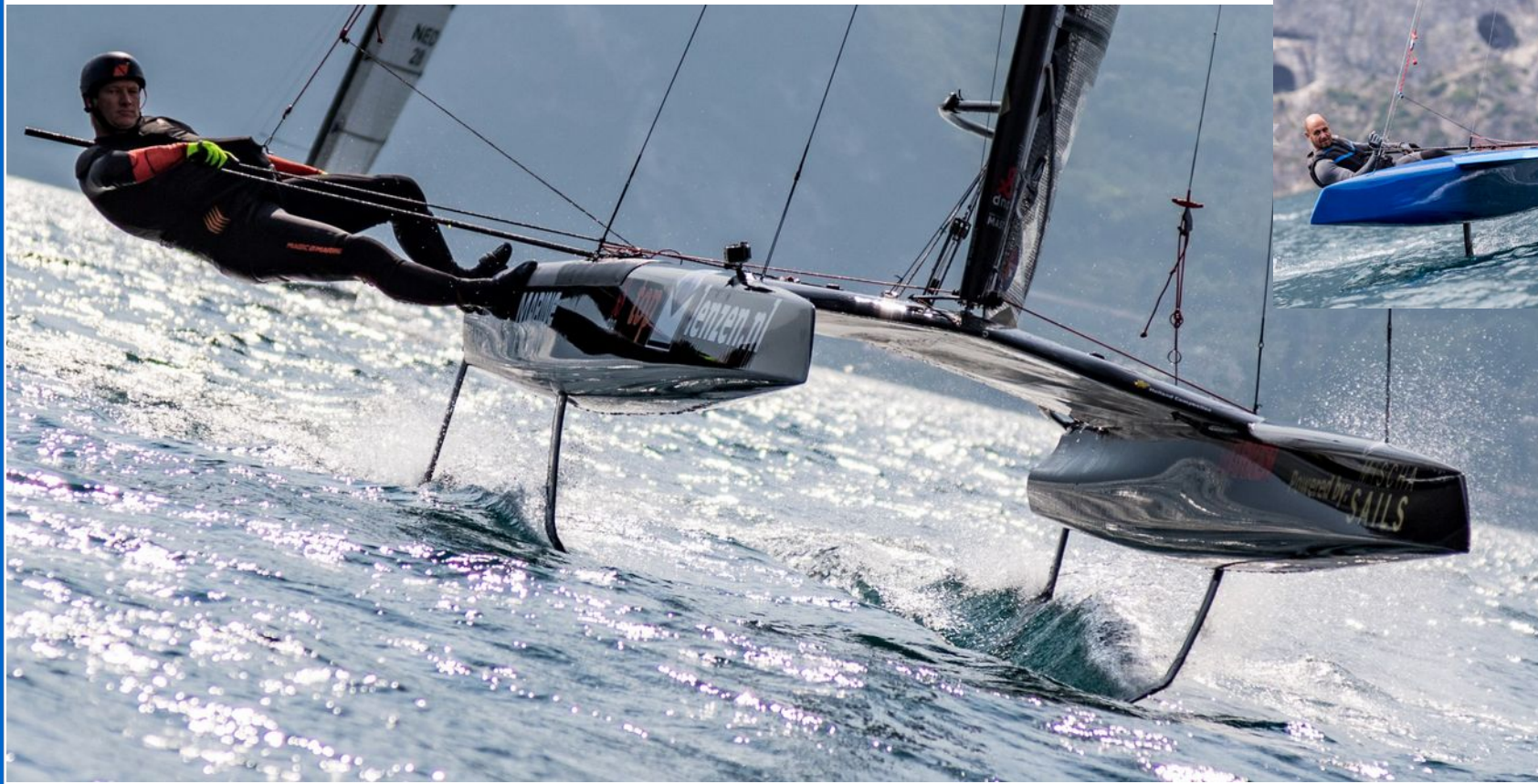
F1 A class catamaran, Australia 2018, LOA 5.49m, 43kg, 13sq meter sail area. 4 Point sail seems to be the configuration of the future catamarans.
