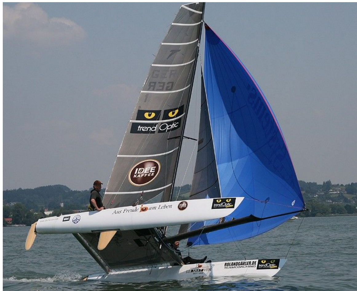
B class Tornado Catamaran, design 1969, first models 1971 ,by Rodney March, Terry Pierce, e Reg White. Olympic Class 1976-2008 It has a jib, a spinnaker, a rotating mast and retractable daggerboards. Note the hull design.
