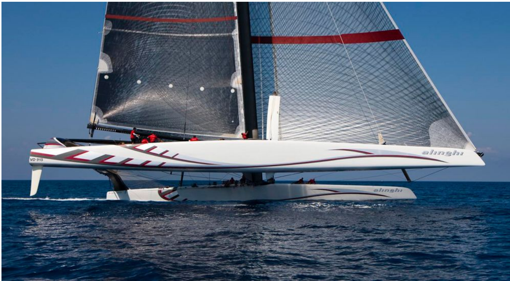
27m Team Alinghi - America's Cup Defender 2007 & 2010. Note the huge Genoa/Code0, and the integrated rudders, the inverted bow, that maximizes speed (at cost of buoyancy/wave stability)
