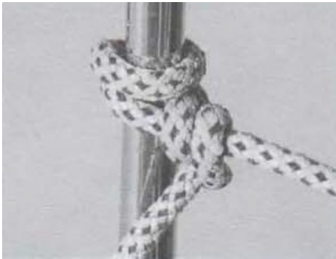
Round turn and two half-hitches
