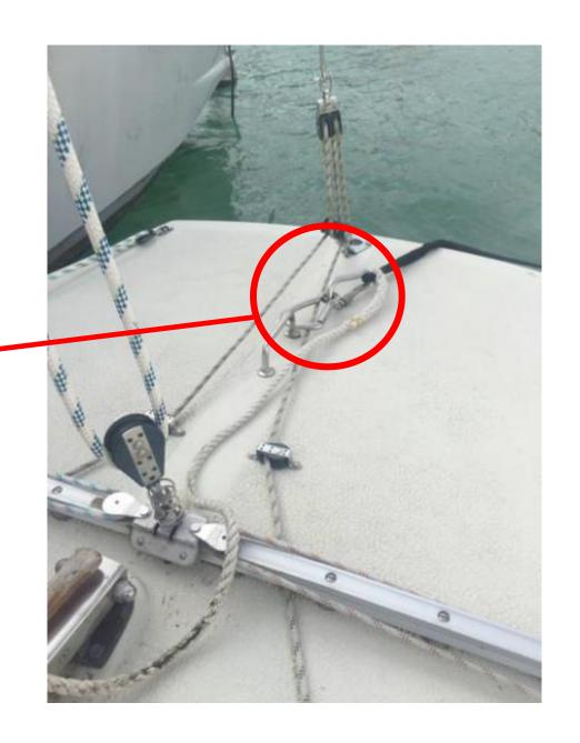
The little cleat screwed to the bottom of the boat is the correct place to attach the fenders.
